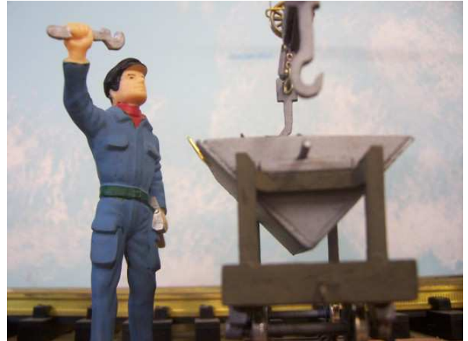
The lifting beam has two hooks that engage with lift pins at the ends of each skip hopper.
