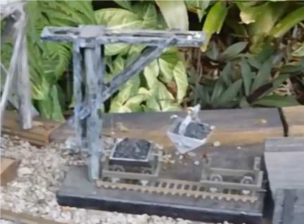
When seated on the trolley, the hooks are released, the skip is moved along ready for the next.
