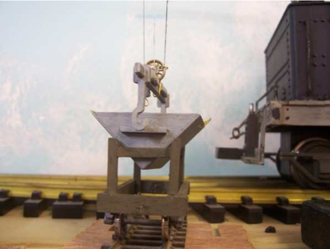
When seated on the trolley, the hooks are released, the skip is moved along ready for the next.
