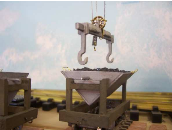
The lifting beam has two hooks that engage with lift pins at the ends of each skip hopper.
